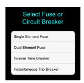
Assuming you have already entered a value for 'amps' in the calculator, selecting one of the four fuses or circuit break types will then perform calculations to determine required fuse size, % multiplier used to determine fuse size (based on NEC 430-52), and also provides the NEC reference. An example output window is shown below:
